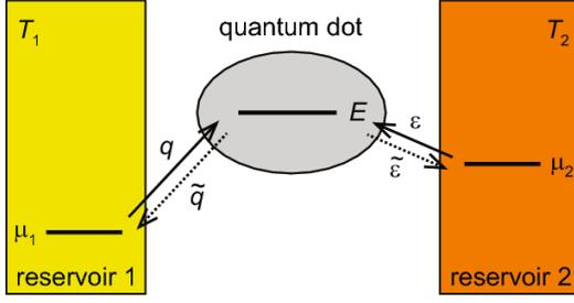
Fig. 2. (Color online) Schematic of the model. There are two reservoirs or leads 1 and 2 with temperatures  $T_1$  and  $T_2$  and chemical potentials  $\mu_1$  and  $\mu_2$ , respectively. An electron can move from one reservoir to the other via the quantum dot, which has a well-defined single energy level  $E$ . The transition rate from reservoir 1 (2) to the dot is  $q$  ( $\epsilon$ ) and the reversed rate is  $\tilde{q}$  ( $\tilde{\epsilon}$ ).
